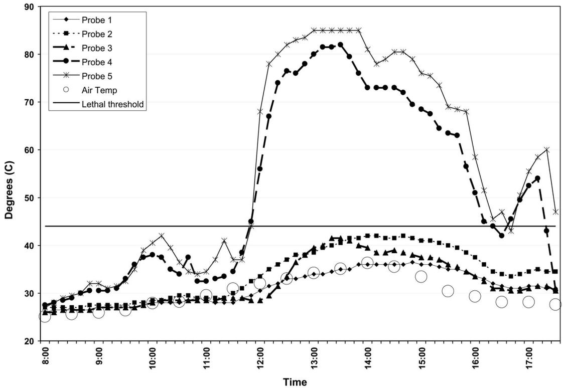
Fig. 1. Data recordings of the temperature loggers on the thin mattress. Loggers 1–3 were placed on the underside, whereas loggers 4 and 5 were placed on the sun-exposed side. The open circles represent ambient temperatures. The line at 44°C is the lethal threshold temperature with a 1-h exposure.
